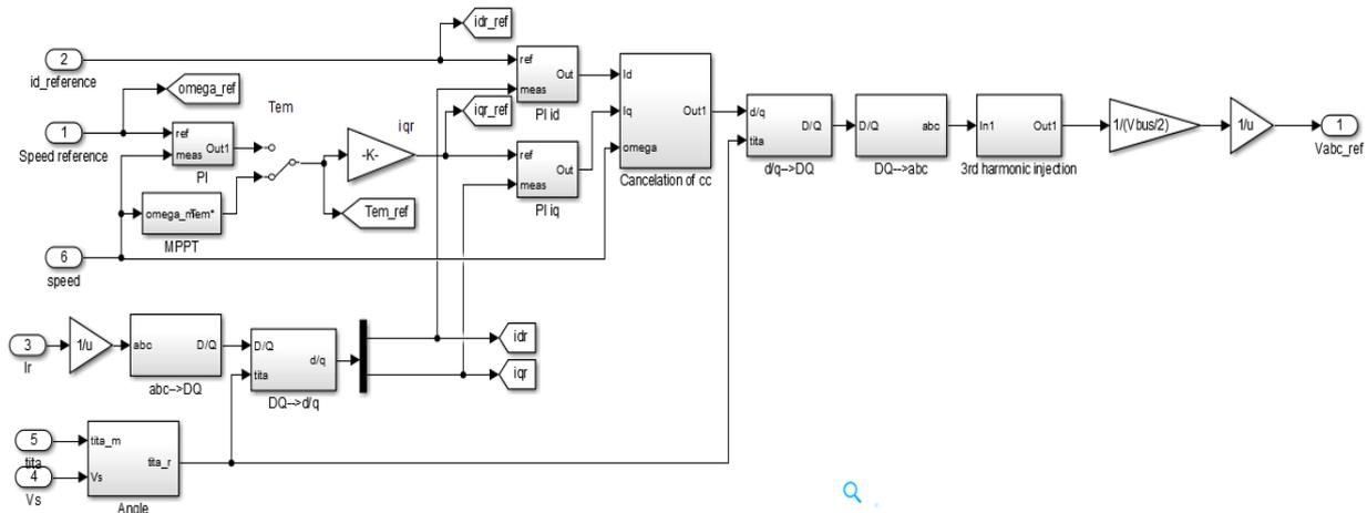
Fig. 2: Simulink Block diagram for rotor-side converter control
