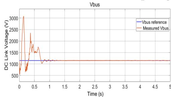
**Fig. 9: DC-link voltage**
