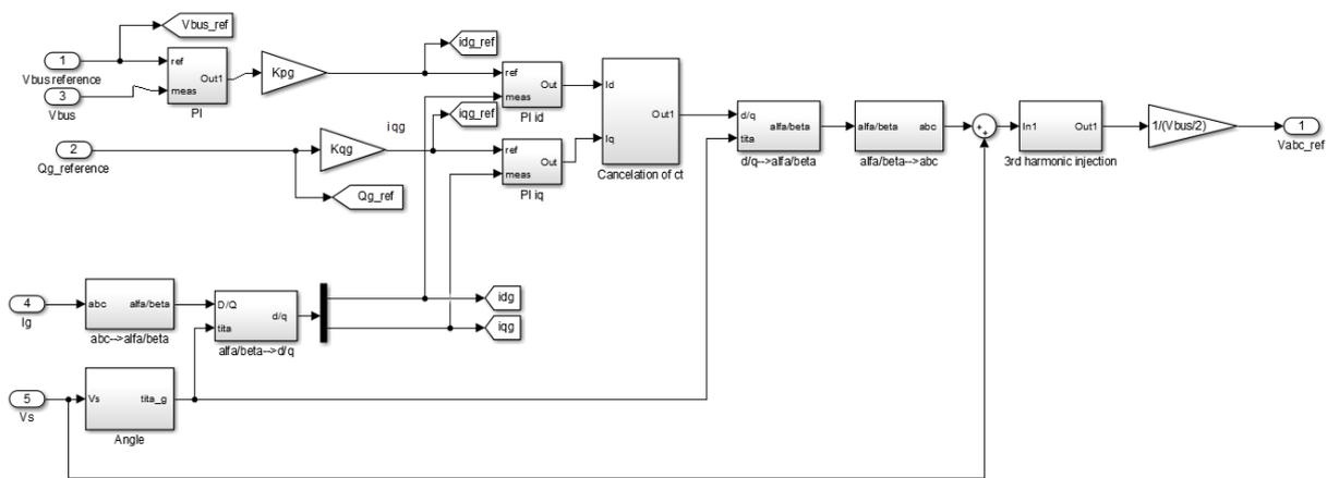
Fig. 3: Simulink Block diagram for Grid-side converter control
