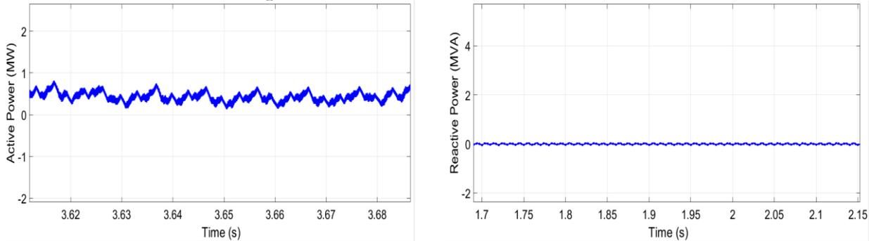
**Fig. 12: Rotor Side Active and Reactive Power Curves**
