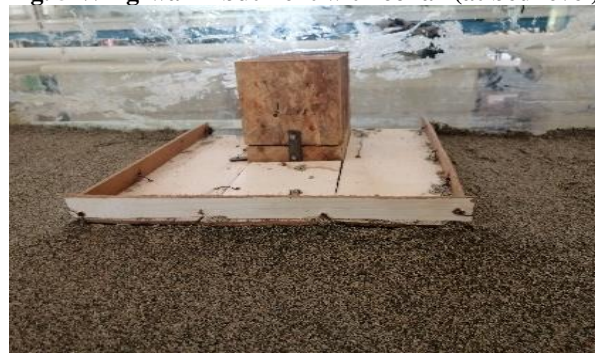
Fig. 6 Vertical-wall Abutment with Hooked-collar (at bed level)
