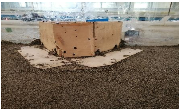
Fig. 4 Vertical-wall Abutment with collar (at bed level)
