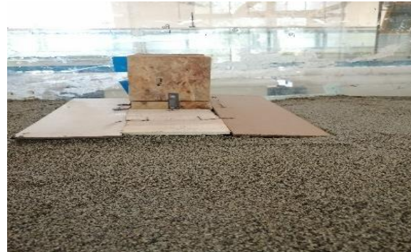
Fig. 5 Wing-wall Abutment with collar (at bed level)
