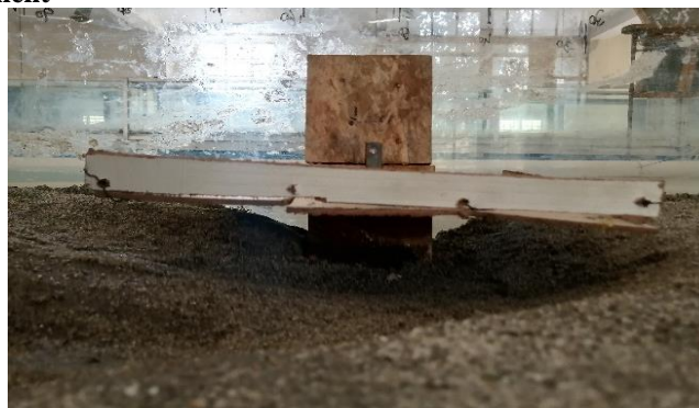
Fig. 10 Scouring of vertical-wall abutment protected with hooked-collar
