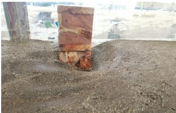
Fig. 8 Scouring of unprotected Vertical-wall abutment
