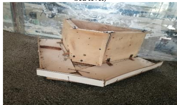
Fig. 7 Wing-wall Abutment with Hooked-collar (at bed level)
