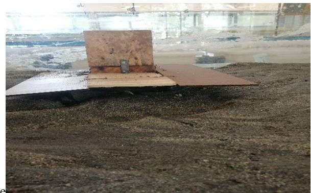
Fig. 9 Scouring of Vertical-wall abutment protected with collar
