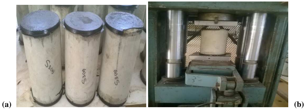
Figure.2. Compressive Strength testing; (a) standard concrete cylinders (b) cylinder under the jaws of UTM
