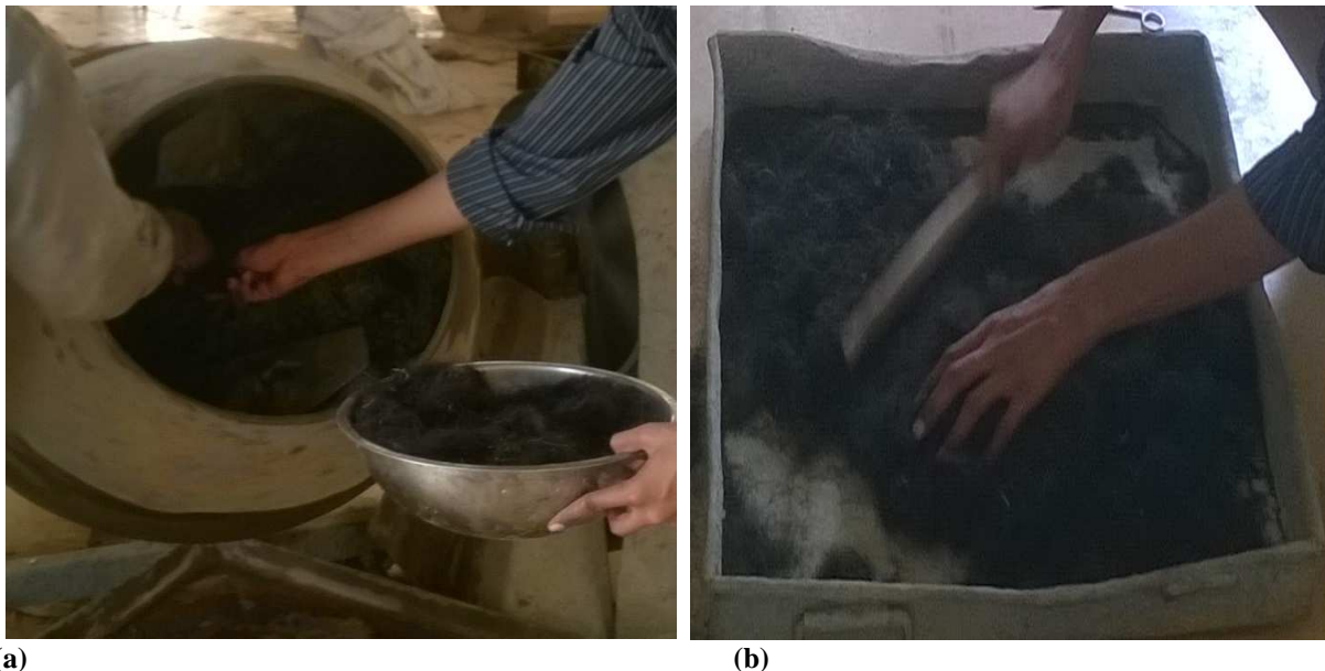
Figure.1. Human Scalp Hair (a) beaten with wooden stick for its separation (b) wet mixing in concrete.
