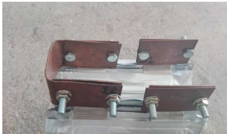
Fig. 6. Parallel and Series Connection of a Stack
