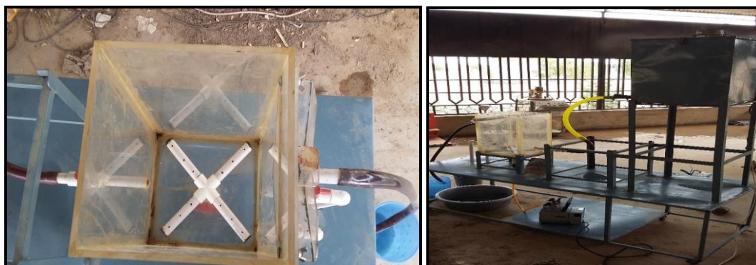
Fig. 2. Dissolved Air Flotation Unit
